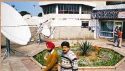
These HNS-built antennas, called very small aperture terminals (VSATs), were installed on the grounds of the Delhi stock exchange in 1997. They are part of a new VSAT network that links member brokers across India to facilitate securities trading. HNS leads the world in installing and operating VSAT networks.
